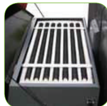
The machine is equipped with large elements separated by polyester fabric for maximum dust filtration capacity.
