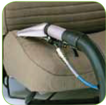
Detergent injection and extraction.
